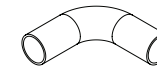
Round Handrail Return Used to create corners and continuous rails around posts. Has two different straight lengths: 4-5/8" for 2" post (marked with a notch) and 5-5/32" for 3" post.
